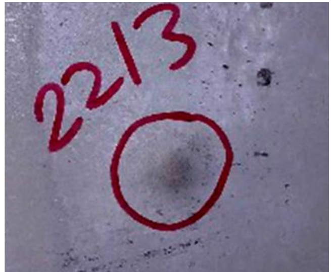
Figure: 12. Back view of the Witness-Plate after 2 shots Result: Accepted
