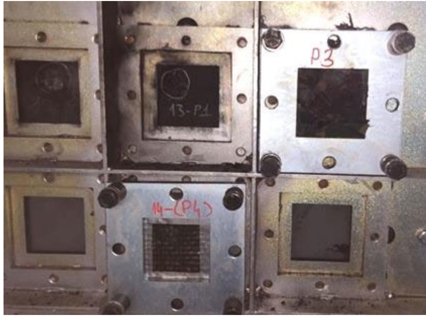
Figure: 27. Target Fixing System of 100 mm x 100 mm Test Panels
