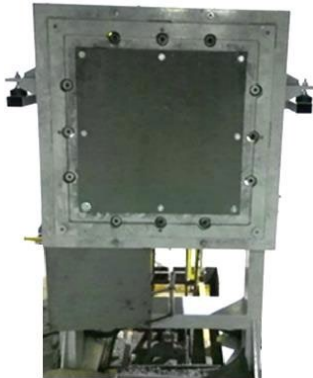
Figure: 25. Target Fixing System of 500 mm x 500 mm Test Panels
